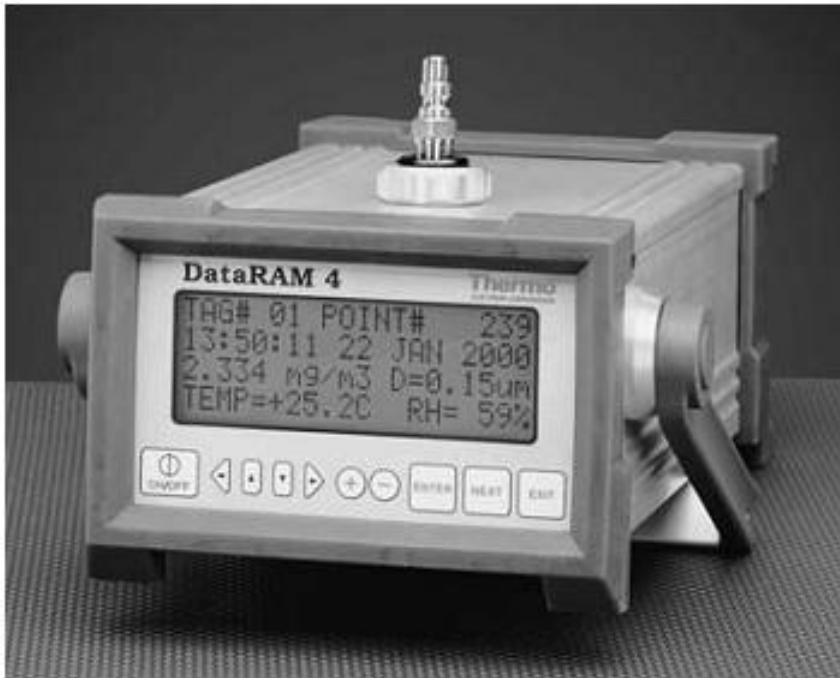
Figure 14.6. Thermo Electron DataRAM-4™ real-time aerosol monitor measures mass concentration while providing continuous real-time readout of both air temperature and humidity. (Courtesy of Thermo Electron Corporation.)
