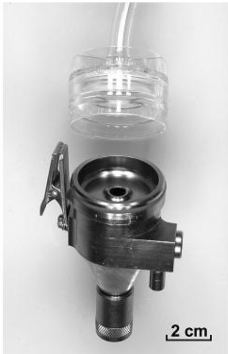
Figure 11.11 GK 2.69 cyclone (BGI Inc., U.S.A.). The sampler may be used for either respirable or thoracic aerosol sampling.
